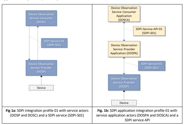
Figure 2a illustrates a SDPi service/use case 01 with service actors (DOSP and DOSC) and a SDPi set of service operations between a device observation service provider (DOSP, actor 1) and a device service consumer (DOSC, actor 2). Figure 2b includes a SDPi service/use case API 01 with service application actors (DOSPA and DOSCA) and a SDPi service API.
