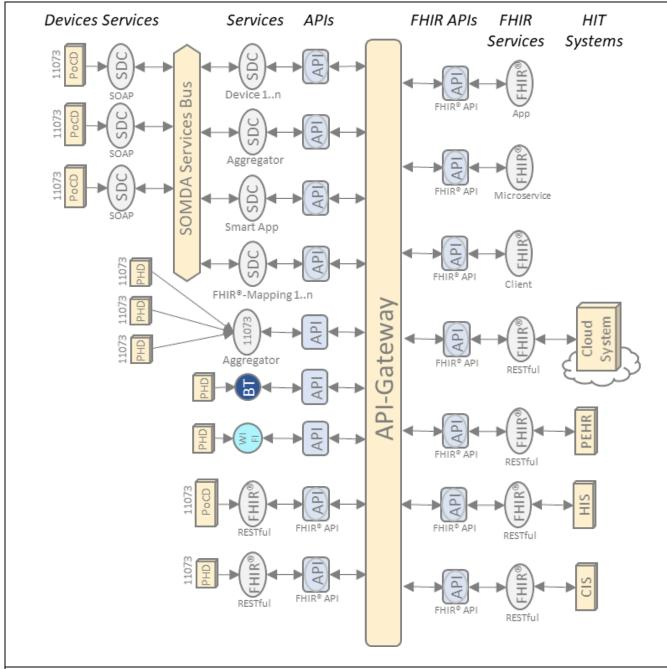
**Fig. 3:** Concept of a generic "system of systems" setup for "Connectathon 4.0" interoperability testing of standards-based service API specifications
